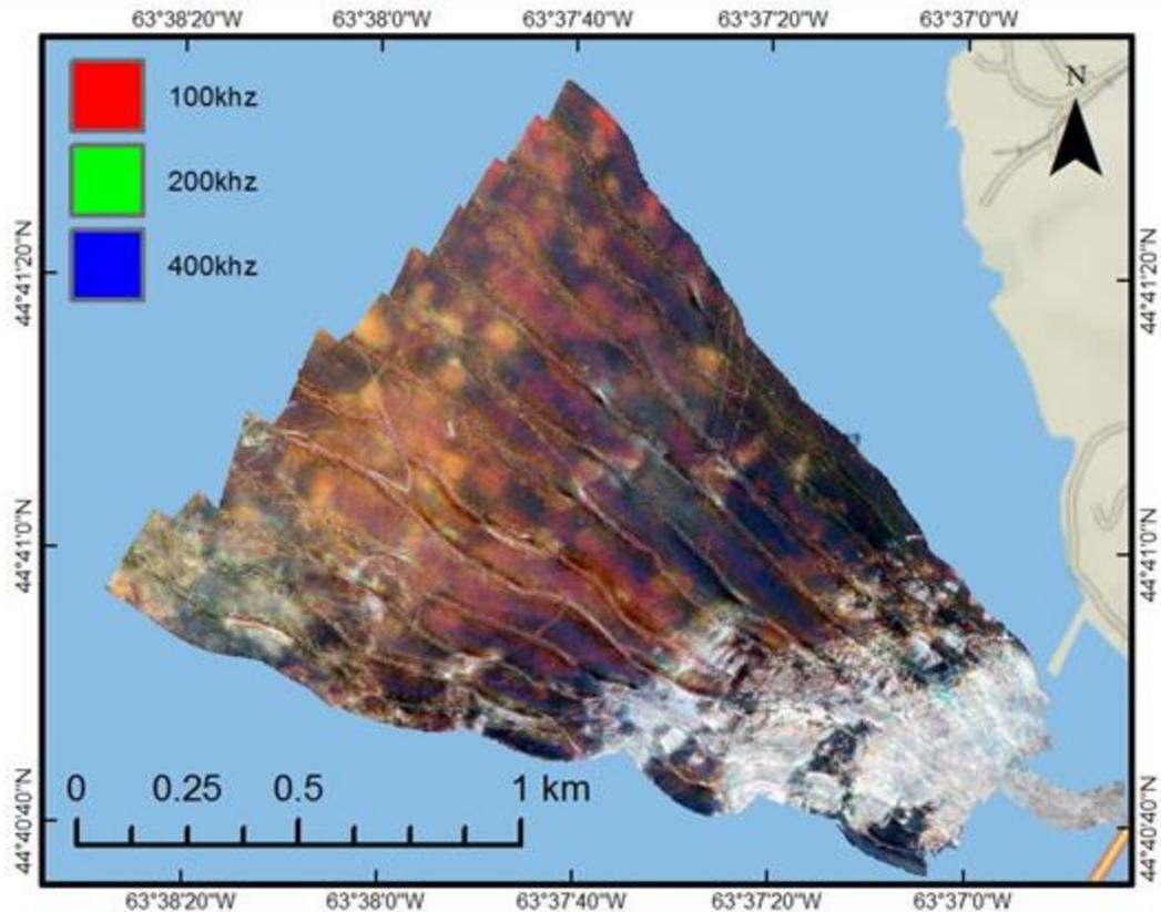
Figure 8: Colour composite image of the multispectral backscatter data.
