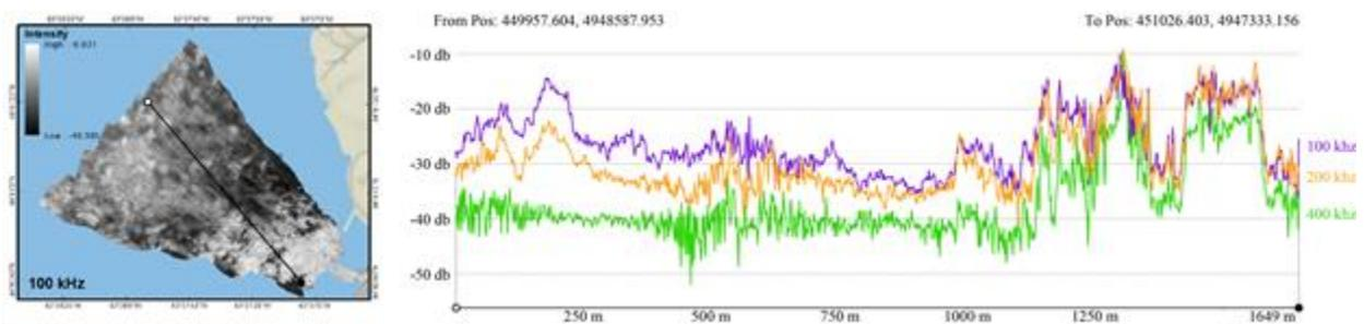
Figure 7: Comparison of differences in backscatter intensities within the survey site between the multispectral mosaics. Backscatter intensities from the three multispectral mosaics are compared along the transect shown on the 100kHz mosaic (left). Backscatter intensities are similar in the hard-substrate region at the mouth of the narrows (SE of the site), and differences are visible in deeper water associated with the dredge spoil deposits.
