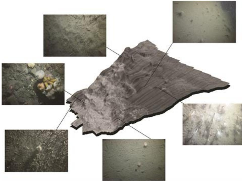
Figure 6: Preliminary ground-truthing underwater imagery from the study site, indicated on the 400 kHz mosaic draped on the bathymetry. Example images shown from different regions of the study site. In the deeper sections of the study site the imagery confirms a soft, muddy seafloor over much of the area, in agreement with the higher frequency backscatter.
