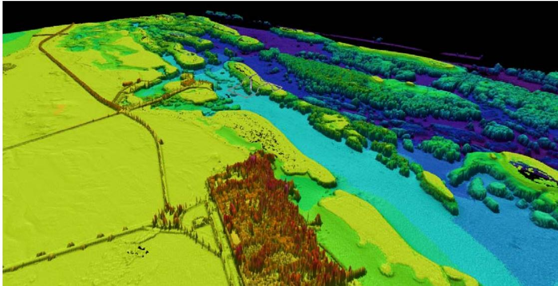
**Figure 2: Charting agencies are increasingly looking for datasets which seamlessly integrate the land-sea interface; this image includes coastal topography, complex nearshore reef structures and deeper navigable channels fused into one deliverable**
