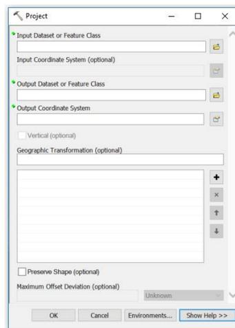
Figure 3. Project Geoprocessing Tool Dialog with Vertical Option
